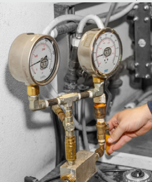
Valves are tested to 1000 PSI and beyond.
